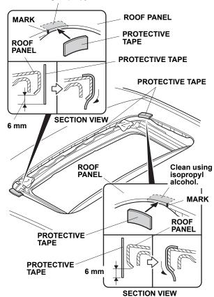
Remove the adhesive backings from two pieces of protective tape, and attach them to the roof panel at the two marks you made. Wrap 6 mm of each protective tape around the bottom lip of the roof panel. Remove the marks. Locate the third indentation from each front corner.
