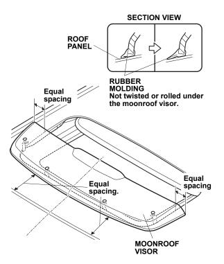
13. Tighten the two screws and two nuts on the sides of the visor first, then tighten the two screws and two nuts on the front. Tighten while applying pressure so there is no gap between the roof panel and the brackets. Torque the screws to 2.0 N·m (1.5 lbf·ft).
