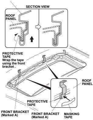
10. Set the moonroof visor on the vehicle roof in front of the moonroof opening, and adjust its position so the holes in the moonroof visor are aligned with the bracket holes. Install the moonroof visor to the front brackets with two screws and two loosely-installed nuts. Remove the masking tape.
