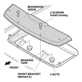
Install the moonroof visor to the side brackets with two screws and two loosely-installed nuts. Remove the masking tape.
