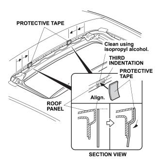
7. Remove the adhesive backing from two protective tapes. Starting at the top edge of the moonroof opening, wrap the protective tapes around the lip of the moonroof opening at the third indentations.
