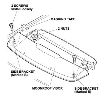
12. Position the moonroof visor with equal spacing on all sides. Check that the rubber molding is not twisted or rolled under the moonroof visor.
